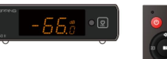
Note: When optical input is selected, ADAT/SPDIF is automatically adapted. In ADAT mode, the default sampling rate is 44.1k/48k, using channels 1+2. For detailed settings, please refer to the user manual.
